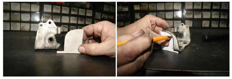
You will need to cut the parts that are marked with an "X" By removing the marked metal it will allow the new VDI hinge to more freely.
