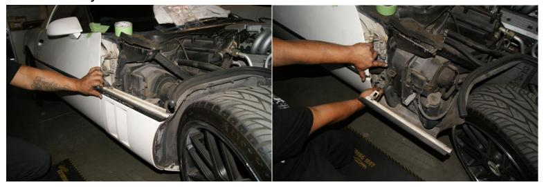
After removing the fender you will have to cut the wire boot bracket as shown.
