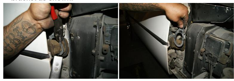
Cut the wire boot in half as shown, do not cut the factory wires.
