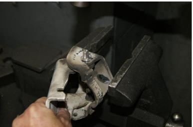
After rounding the flats use a hammer to knock the pin off the hinge.
